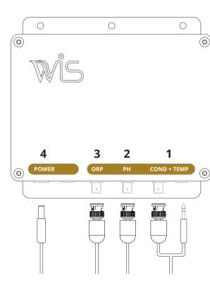
Connect the sensors to the control box
